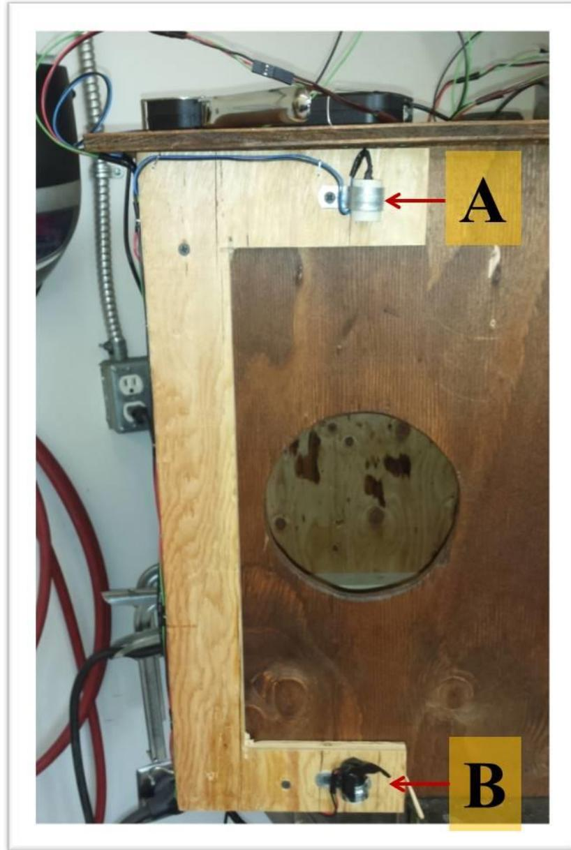
**Figure 3.8.** Photo of (A) photo resistor and (B) laser diode mounting on a Barn Owl nest box, both of which are held with foam inside small pieces of PVC pipe.
