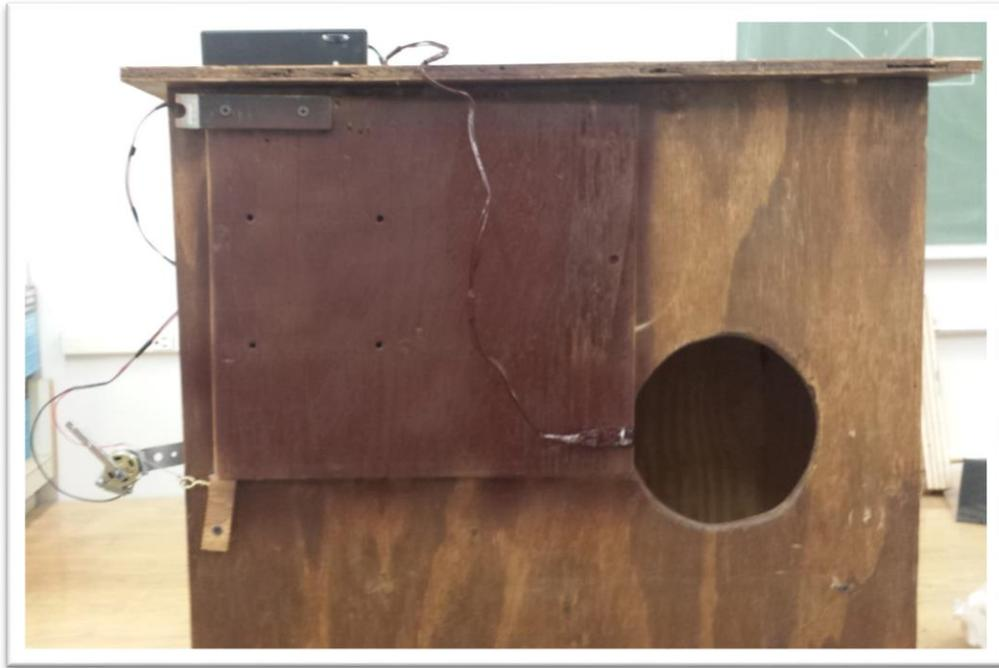
**Figure 3.6.** Nest box with laser-triggered trap door installed. To the bottom left is the trigger mechanism and wooden peg used to hold the door open. The small black box on top of the box holds the Arduino Nano microprocessor and associated wiring. On the top left of the trap door is the weight used to adjust the center of gravity of the trap door so that it appropriately swung to cover the entrance.
