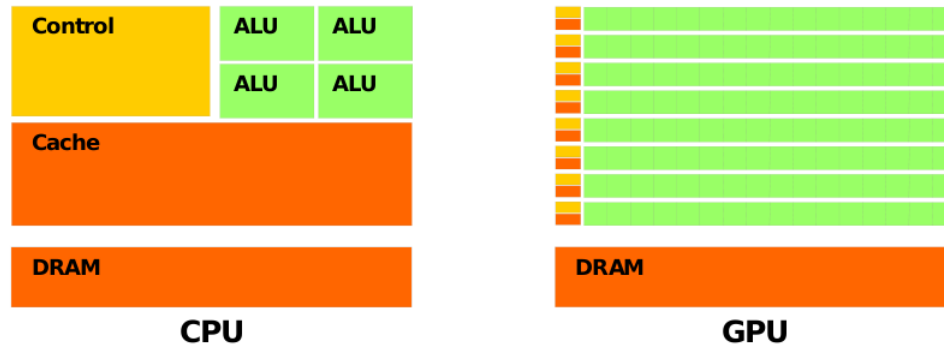
Figure 2.8: CPU and GPU fundamental architecture design. [19]
