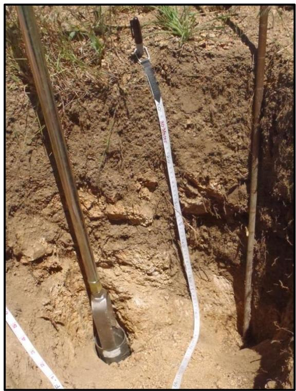
Figure 2.2 Example of penetration rod and auger piercing the upper darker, finer-grained mobile regolith, and set into the underlying coarser immobile regolith (granodiorite). The methods yielded similar results when tested side-by-side.
