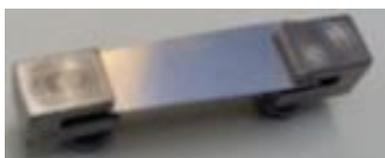
**Figure 27: LSR thin film adapters**
