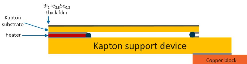
**Figure 23: Parallel thermal conductance set-up with  $\text{Bi}_2\text{Te}_{2.8}\text{Se}_{0.2}$  film**
