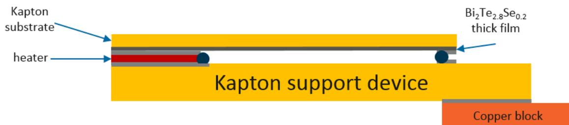
**Figure 24:** Revised parallel thermal conductance set-up with  $\text{Bi}_2\text{Te}_{2.8}\text{Se}_{0.2}$  film
