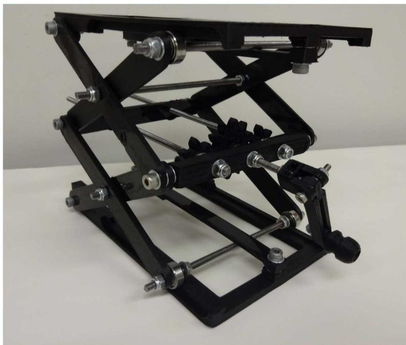
**Figure 1.2** Open-source lab jack with 3D-printed parts. Reproduced under terms of the Creative Commons Attribution License from [8].
