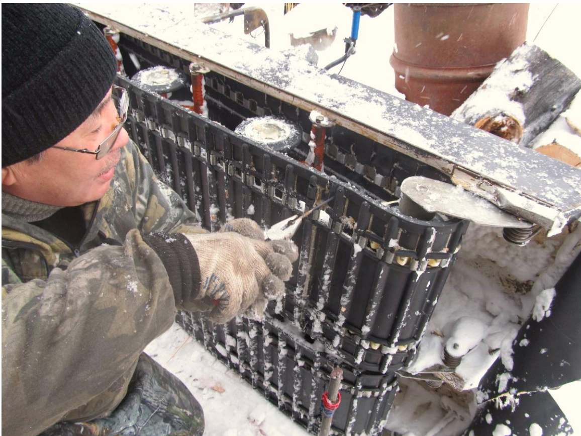
Picture 7.1 Sewing tear in snowmobile track with hot nail and wire
