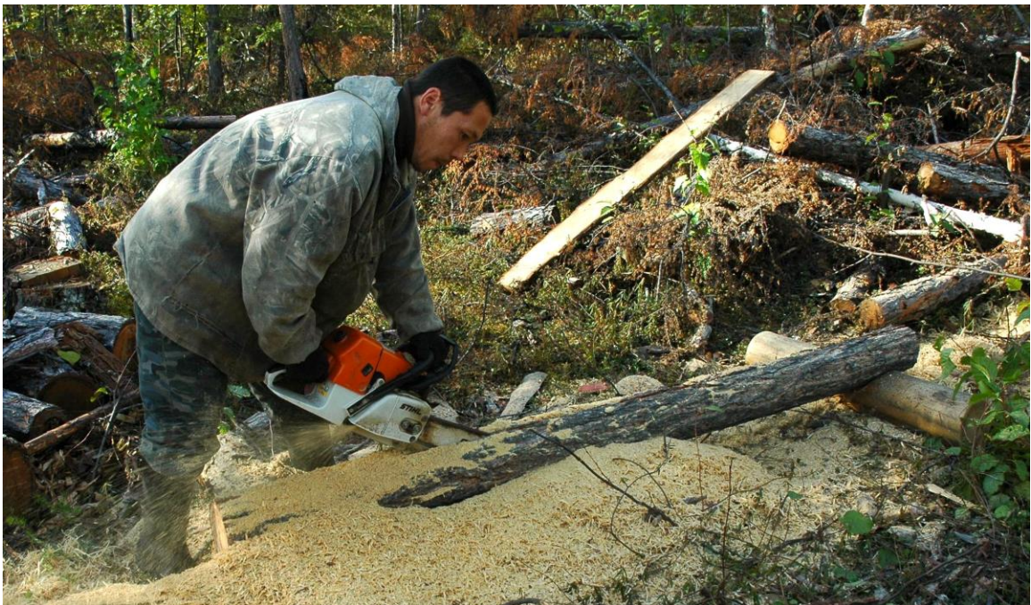
Picture 6.17 Ripping boards with a Stihl 660 chainsaw
