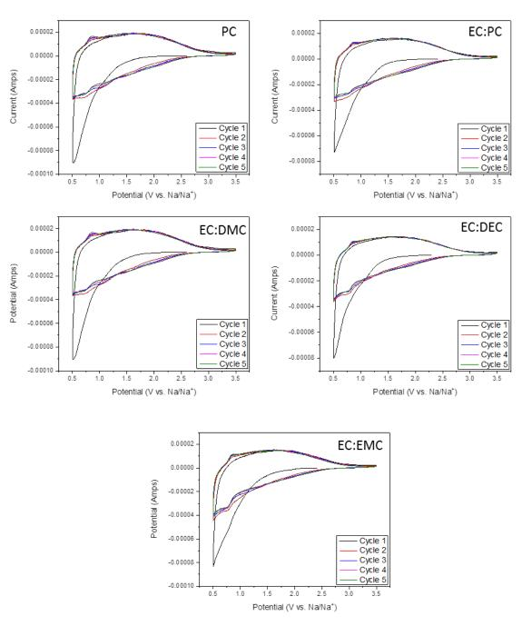
*Figure 7* Cyclic Voltammetry Data, all electrolytes tested are reported here.
