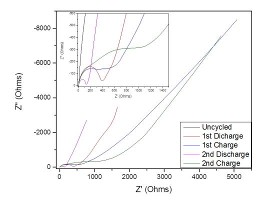
*Figure 13* EIS measurements for half-cell with EC:DEC electrolyte. The insert shows the origin with greater detail.
