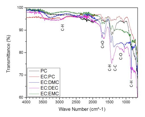
*Figure 14* FT-IR spectra for the electrodes after one complete discharge/charge cycle for each of the electrolytes tested.
