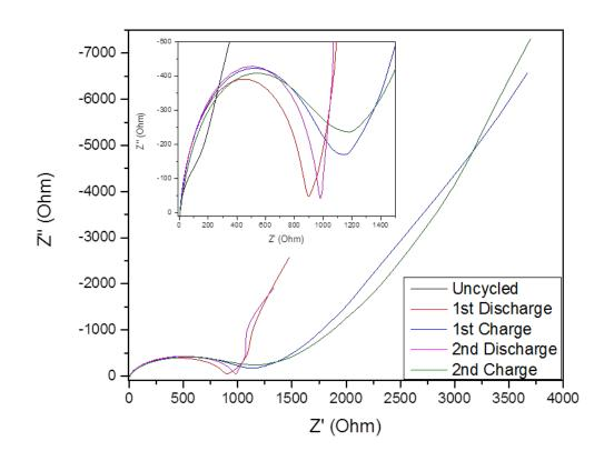
*Figure 9* EIS measurements for half-cell with PC electrolyte. The insert shows the origin with greater detail.
