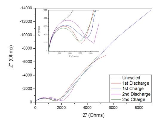
*Figure 10* EIS measurements for half-cell with EC:PC electrolyte. The insert shows the origin with greater detail.
