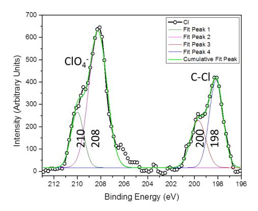
*Figure 17* XPS data from half-cell with PC electrolyte, focused on the Cl spectra collected. The black line and circles shows the data collected by the XPS. The fitted peaks 1-4 are the identified peaks in the spectra and the cumulative peak fit in green shows that the fit matches the data.
