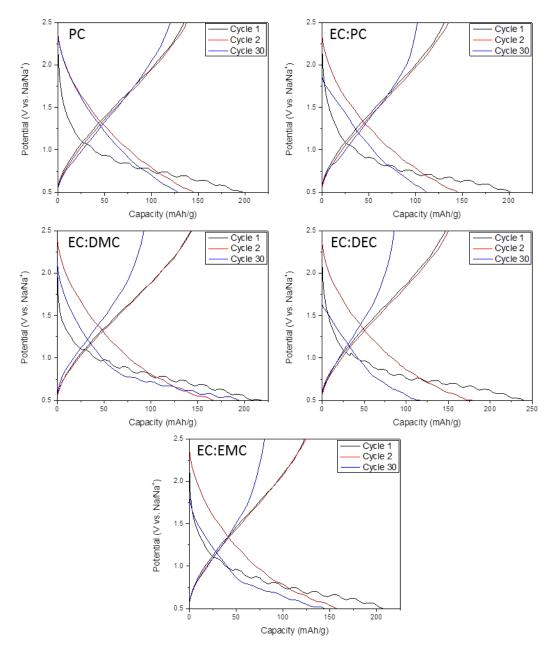
*Figure 6* Voltage profiles of the measured electrochemical performance on cycling the half-cells. Displayed are the 1<sup>st</sup>, 2<sup>nd</sup>, and 30<sup>th</sup> cycles. All electrolytes tested are reported here.
