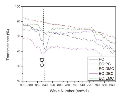
*Figure 15* FT-IR data at low wavenumbers. The dotted linemarks the C-Cl bond.
