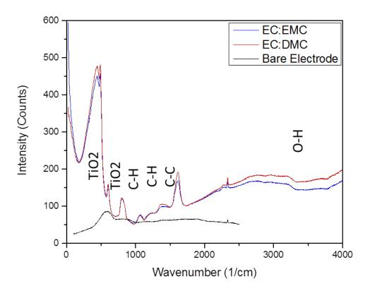
*Figure 16* Raman spectra for TiO2 electrodes in charged state. Two electrolytes were tested, EC:EMC and EC:DMC.
