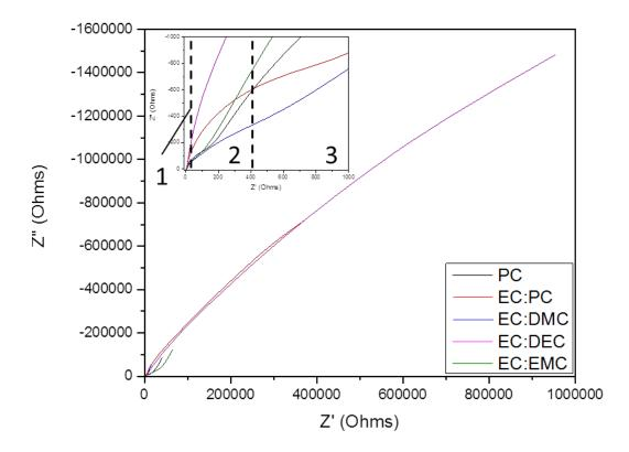
Figure 8EIS measurements of the uncycled half-cells. Insert shows the originin greater detail. Section 1 is the high frequency region. The high frequency regiondescribes the behavior of the bulk electrolyte. Section 2 is the medium frequencyregion. The medium frequency region shows the interface and interface reactions.Section 3 is the low frequency region, which indicates the diffusion in the solidelectrode.
