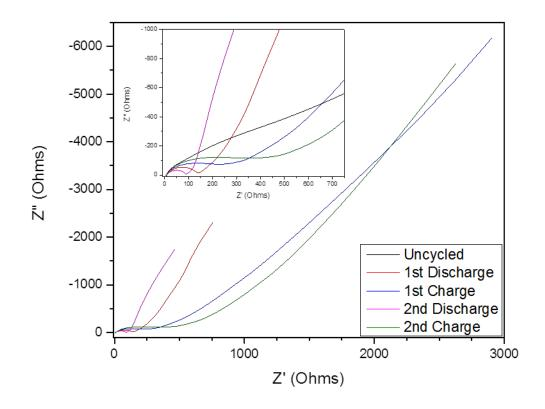
*Figure 12* EIS measurements for half-cell with EC:DMC electrolyte. The insert shows the origin with greater detail.
