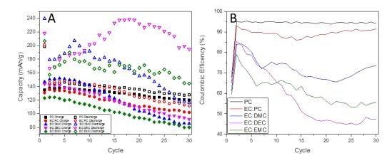
*Figure 5* Half-cells of TiO<sub>2</sub> NTs vs Na/Na<sup>+</sup>. A) Electrochemical capacity of the half cells. B) Coulombic efficiency of the half cells.
