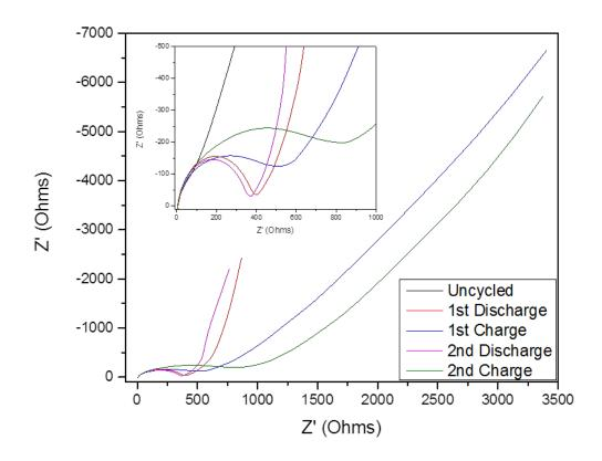
*Figure 11* EIS measurements for half-cell with EC:EMC electrolyte. The insert shows the origin with greater detail.
