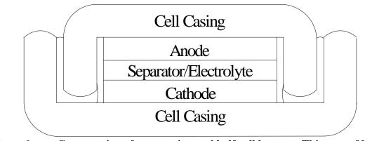
*Figure 1* Cross-section of an experimental half-cell battery. This type of batter was utilized in the current work.
