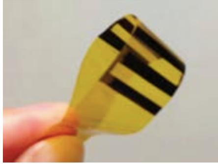
**Figure 9. Ink-jet printed thermoelectric device on Kapton [54]**
