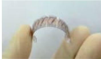
**Figure 11. TEG screen printed onto a glass fabric [22]**
