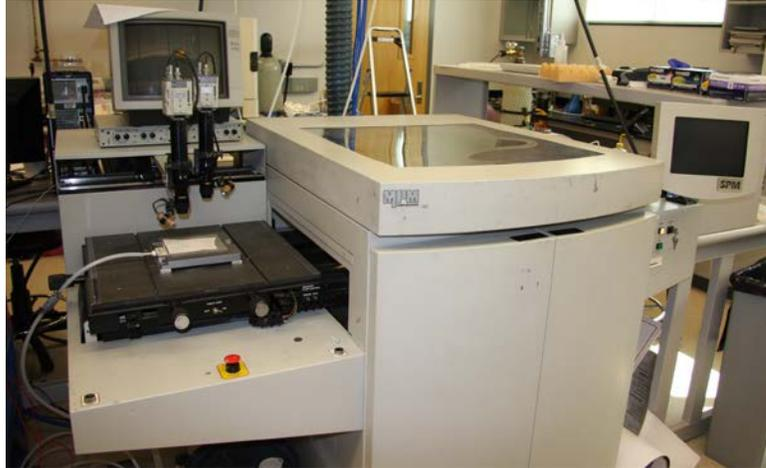
**Figure 13. MPM SPM screen printer**
