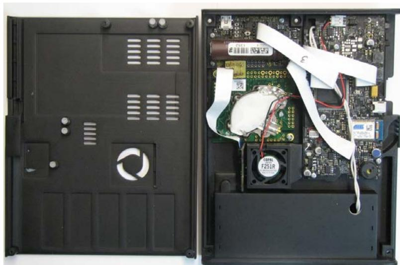
**Figure 4:** Full PMON Unit, Top Removed
