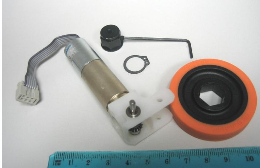
**Figure 4.6 Motor, Hub, and Wheel Disassembly**
