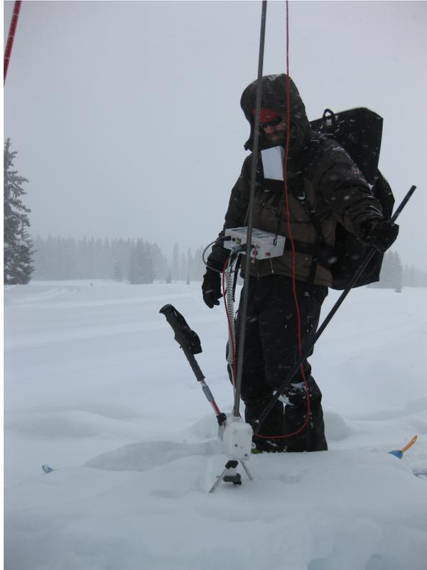
Figure 1.2: The Snow Micro Penetrometer being used to evaluate snowpack layering.
