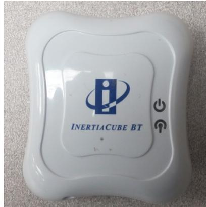
**Figure 1: Inertial Measurement Unit**
