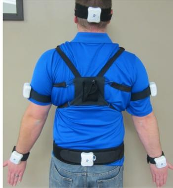
**Figure 2: IMU devices on participant**
