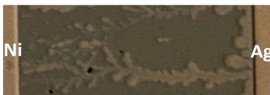
**Figure 4.15** Electrochemical growth of the Ag dendrite in the Ag-Ge-Se electrolyte [166]
