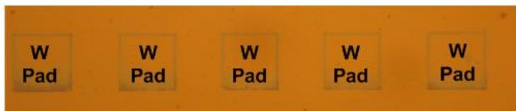
**Figure 3.10** W pad formation top view on the sample
