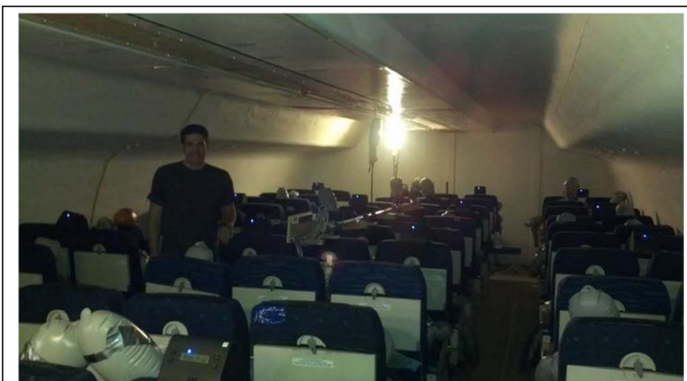
**Figure 120** Interior of the aircraft cabin mockup with WAQM sensors in place. The blue LEDs on the sensors are visible on the seat headrests.
