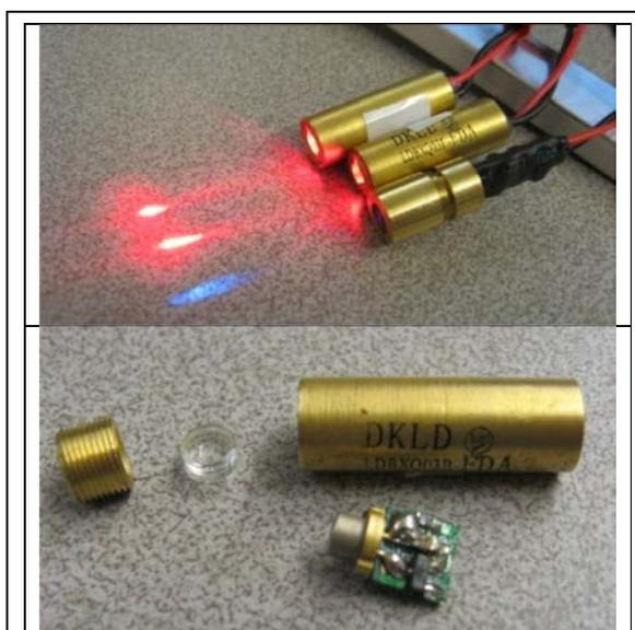
**Figure 27** Laser modules evaluated during WAQM OPC development. At top are three of the modules considered for prototype development. At bottom is a dissected module of the type deployed in the WAQM OPC.
