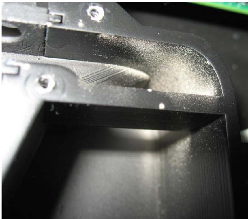
**Figure 104** Inertial deposition in a bend in the WAQM OPC flow channel. This bend occurs after the photodiode, but illustrates particulate impaction when the air velocity changes direction. The particulate matter builds up in the channel after running continuously for many weeks.
