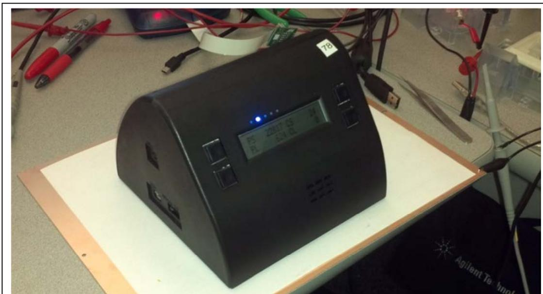
**Figure 18** Testing noise coupling on a grounded copper sheet. The WAQM OPC unit is powered through a two-prong wall transformer with isolated ground.
