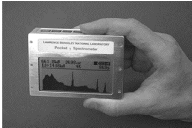
Figure 12 Pocket size CdZnTe detector [20] © 2005 IEEE.
