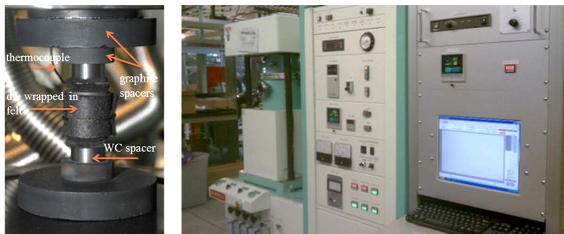
Figure 4 Sintering chamber die set up with felt wrapped around graphite die and tungsten carbide spacers (left). Pulsed electric current sintering machine at CAES in Idaho Falls, Idaho (right).
