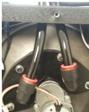
Figure 4.4 Added Exhaust Plate and Hosing
