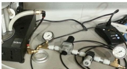
Figure 5.6 Alternate Air Supply In-Line Structure
