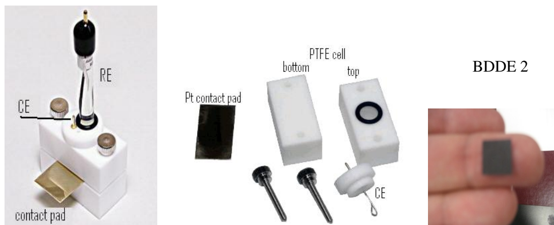
Figure 2.2 This figure shows the minicell fully assembled and ready for use in the far left panel. The connection pin is shown for the counter electrode as well as the RE6 reference electrode protruding from the top of the cell. The center panel shows the individual components in an exploded view. The far right panel shows the BDDE on my hand for perspective. Either a Pt or BDD working electrode was used in the minicell.
