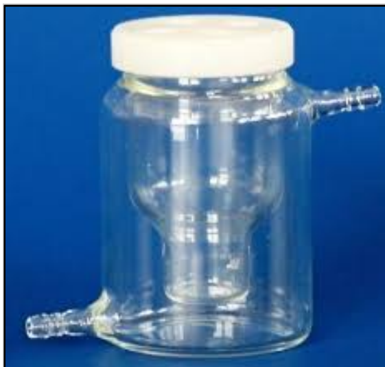
Figure 2.4 A typical jacketed rotating disk electrode cell. This image (courtesy of BASi) is a small volume three electrode cell with gas purge holes in the PTFE lid. The total volume for this cell is 25 mL with a 10 mL well.
