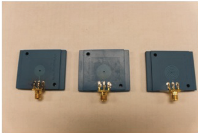
Figure 3.2: The three ICP antenna designs tested: \alpha , \beta , and \gamma . The designs vary in diameter, pitch, and number of turns. [41]
