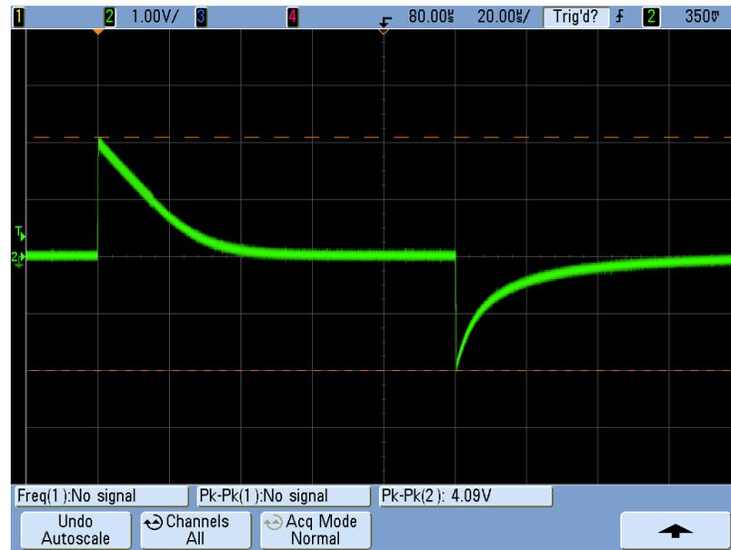
Figure 3.13: Frequency response of a  $100\mu\text{s}$  pulse
