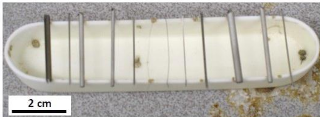
Figure 6: An optical image representing the placement of the titanium wires of different diameters over the alumina boat for carrying out oxidation in the high temperature tube furnace.
