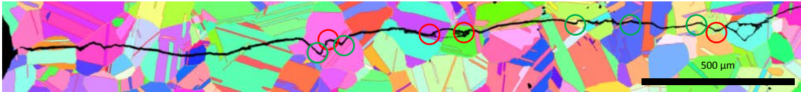
Figure 29. IPF map showing examples of well-defined crack path changes (green circles) and those with less definition (red circles). Only a small selection of crack path deviations is marked
