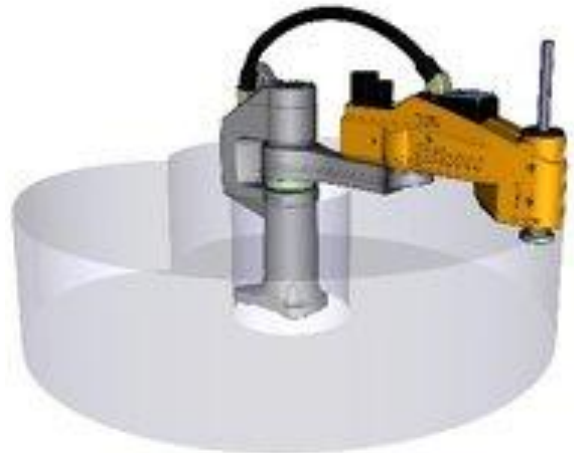
Figure 3. SCARA Work Envelope 2D [42] Figure 4. SCARA Work Envelope 3D [41]
