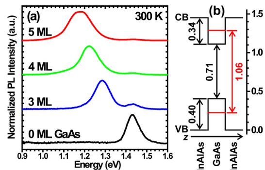
Fig. 1. (a) Room temperature PL from GaAs/In<sub>0.52</sub>Al<sub>0.48</sub>As(111)A QDs grown with different deposition amounts from 0 ML (i.e., control with no QDs) to 5 ML. (b) Band diagram for GaAs(111)A QDs under 3.8 % biaxial tension. Calculated ground state emission for a 4 ML GaAs QD is in red. All values are in eV. Reprinted from [9], with the permission of AIP Publishing.
