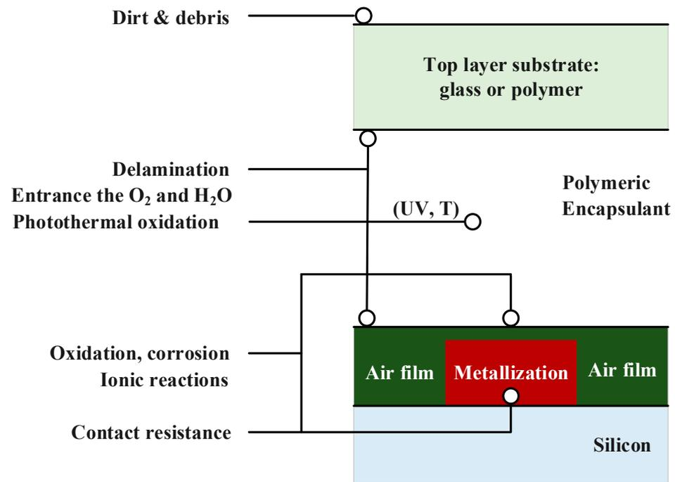
**Figure 6.** PV degradation process through delamination [89].
