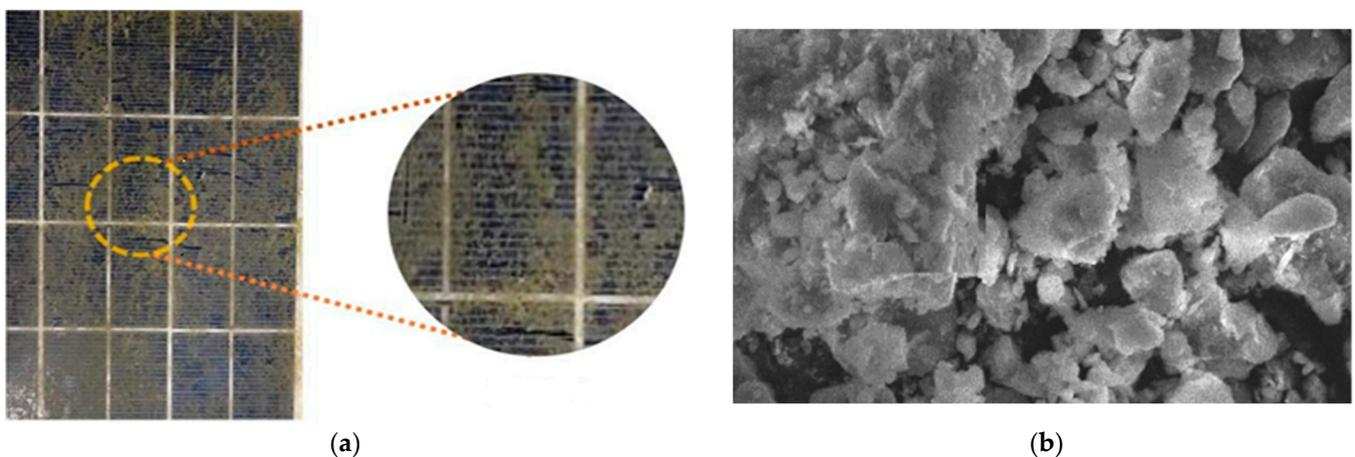
**Figure 2.** (a) Accumulation of dust on the PV surface and (b) microscopic view of the accumulated dust (this figure was developed from the original sample and experiments that were carried out in the laboratory).
