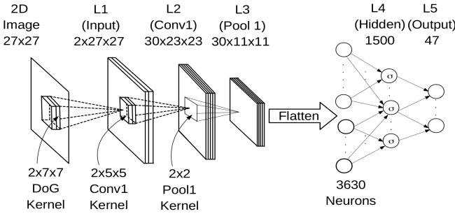
Fig. 1. Proposed SNN architecture. Here, layers  $L_1 - L_3$  are the feature extraction layers and layer  $L_3 - L_5$  are the feature classification layers.
