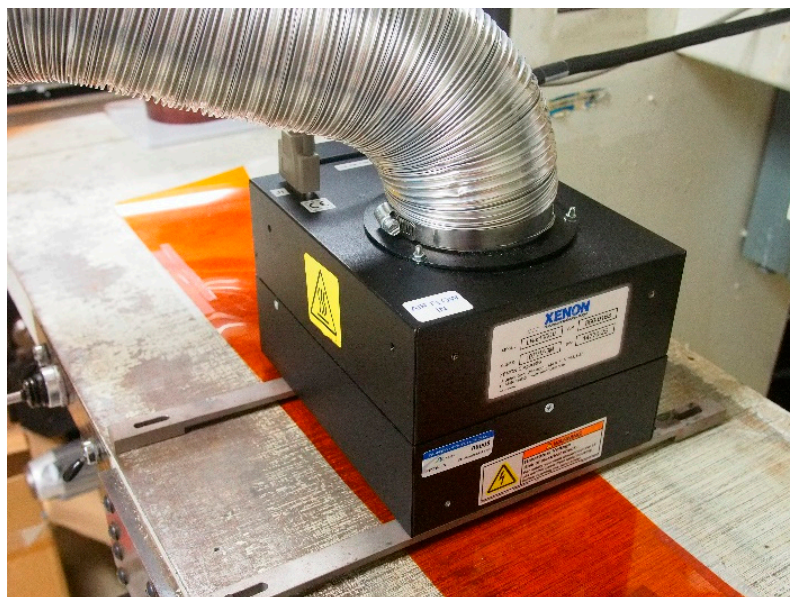
Figure 1. Xenon Sinteron-2000 system used for developing the CNT ink.
