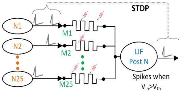
**Figure 2: Memristor-based neural network used in this study. 25 pre-synaptic neurons are connected to one post-synaptic leaky integrate-and-fire neuron via single memristors. The network uses shaped pulses to achieve pair-based STDP for pattern learning.**
