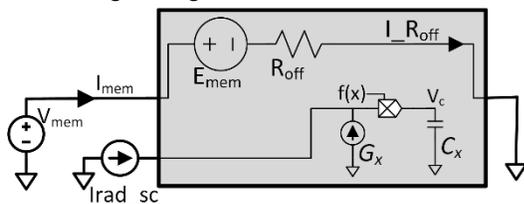
**Figure 1: Non-linear drift memristor model implemented in Cadence Virtuoso Spectre. State-altering radiation ( $I_{rad\_sc}$ ) is added to the auxiliary circuit so it can modify the state of device instantaneously.**
