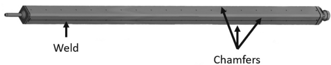
Fig. 1. Rendering of TREAT's unique fuel cladding assembly, which includes chamfered corners and welded end caps.
