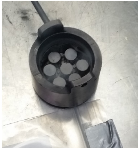
Fig. 2. Green U_3Si_2 pellets loaded into the graphite sintering crucible, before sealing in an inert atmosphere glovebox.
