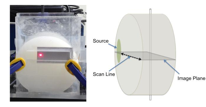
Figure 5.1: (a) Photograph of experimental setup, with the scan line shown. (b) 3D perspective view of phantom setup with 2D image plane shown.
