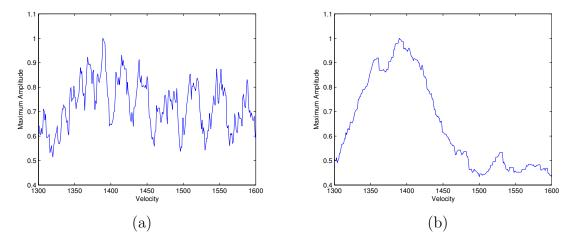
Figure 6.7: Maximum amplitude of LU wave in Trial 2 (a) and PA wave in Trial 3 (b) for a given velocity. The velocity of sound in the phantom for optimum NMO correction was 1390 m/s.
