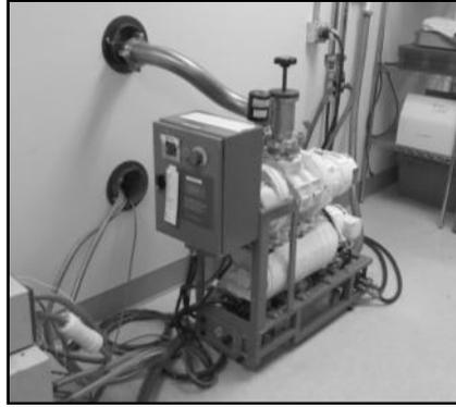
**Figure 75: Two-Stage Mechanical Vacuum Pump**
