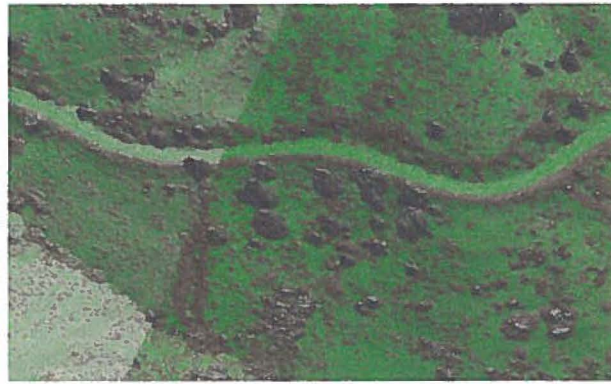
Figure 4b: Green points are ENVI classified ground points using BCAL tools and a 4 m canopy spacing, cleaned using Steps 1 – 10, with the addition of all points within 10 cm of the interpolated surface. Background DEM is the interpolated surface of all points.
