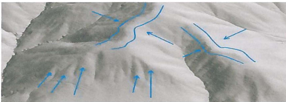
Figure 1c: Accurate representation of topographic features using 2.5 meter canopy spacing to classify points in areas with rapid slope transitions.
