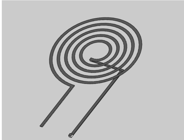
Figure 3. 3D solid model of antenna coil as seen in SolidWorks.
