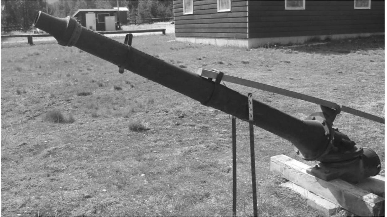
**Picture 4: A nozzle from a hydraulic giant, a leftover from the era of hydraulic mining, where high pressured water was used to erode the gold bearing gravel from the hillside, a mining method that was used mostly in lower Warren Meadows.**
