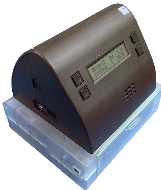
Figure 10 IHAQ Monitor Atop the External Battery Enclosure.
