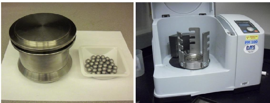
**Figure 15. Milling vessel and media (left) and PM100 planetary ball mill (right)**
