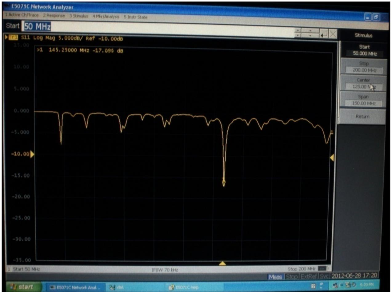
**Figure 28**  $S_{11}$  (dB) of the medium when using a loop coupling.
