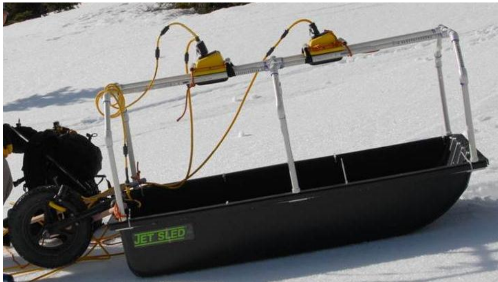
Figure 4.2 Photograph showing sled with radar. GPR antenna are suspended 0.7 m above the snow surface on a PVC framework attached to a sled.
