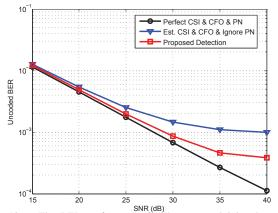
Fig. 12. The BER performance for the proposed joint data detection algorithm at  $\sigma_{\Delta}^2=10^{-4}{\rm rad}^2$ .
