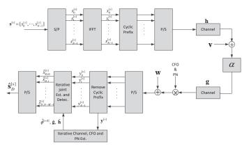
Fig. 2. Illustration of transceiver structure of the OFDM relay system.
