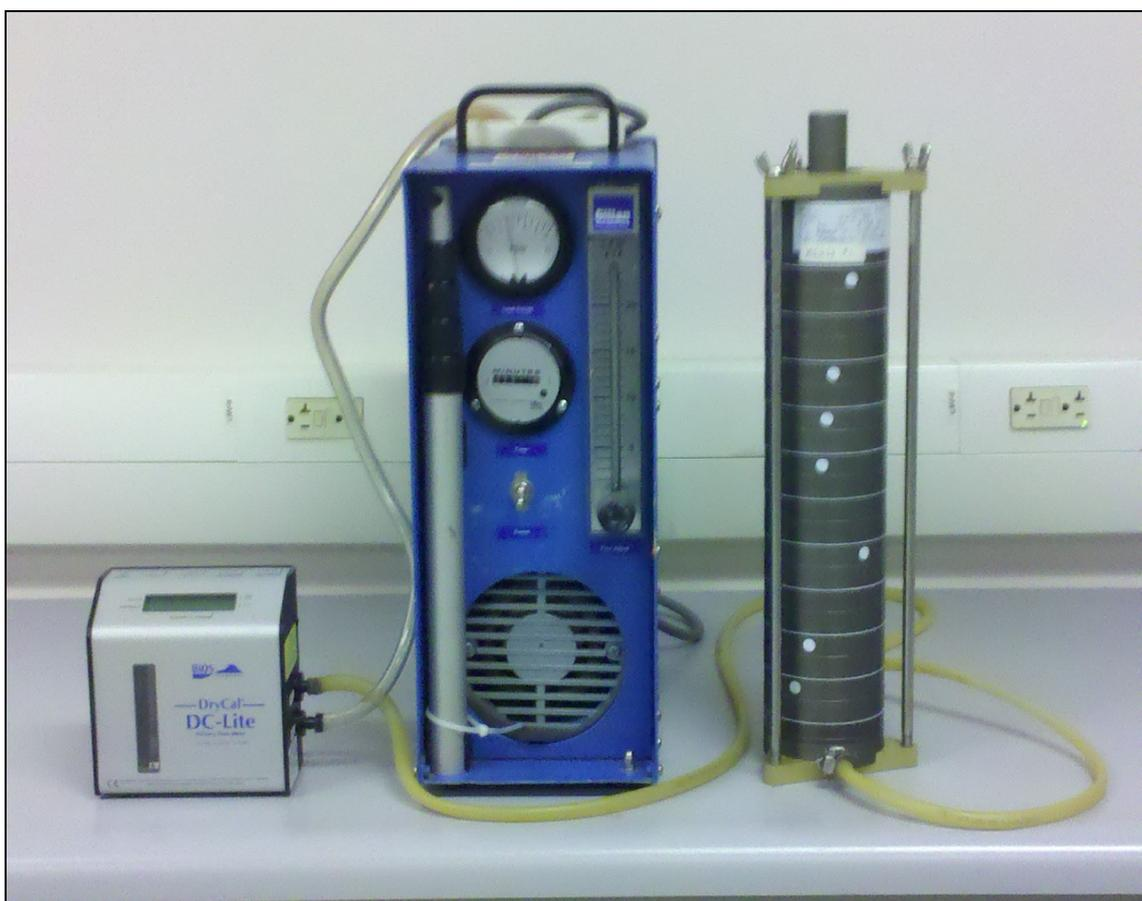
**Figure 5** BIOS DryCal Air Flow Meter, Aircon 520 Air Sampling Pump, and MOUDI
