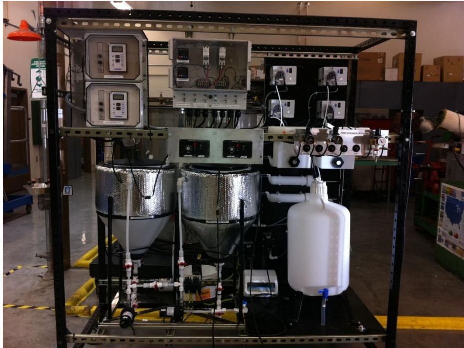
Figure 2.3. The Pilot Scale Integrated Nursery Reactor (left) and Hydrolysis Reactor (right) System.
