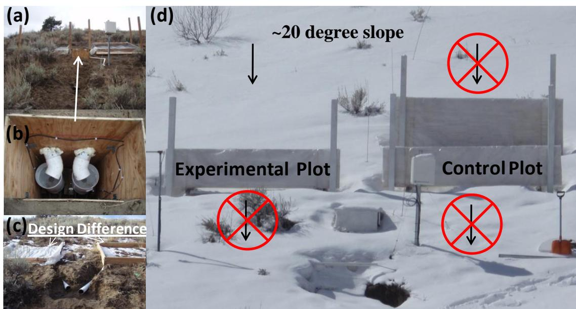
**Figure 4. Paired lysimeter experiment photos. (a) Shows the paired lysimeter experiment prior to snowfall. (b) Shows the tipping buckets and plywood housing. (c) Highlights the design difference on the upslope edge of the two plots. (d) Shows the completed experiment during winter.**
