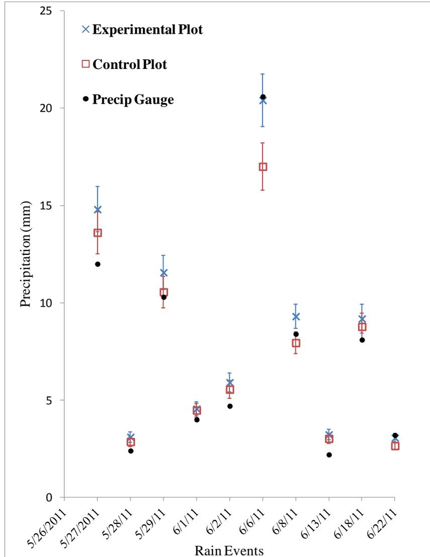
**Figure 10. Paired lysimeter experiment June-July rainstorm collection efficiency comparison.**
