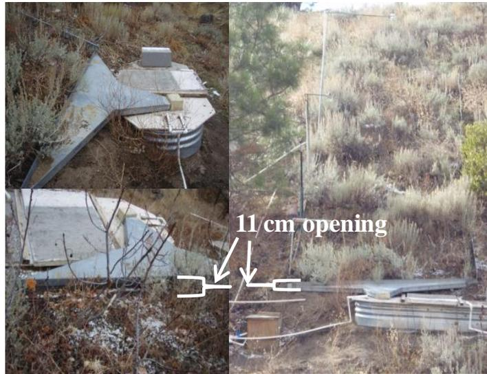
**Figure 2. Overland flow runoff plot. The plot collects water moving along the ground surface or in the bottom 11 cm of the snowpack.**
