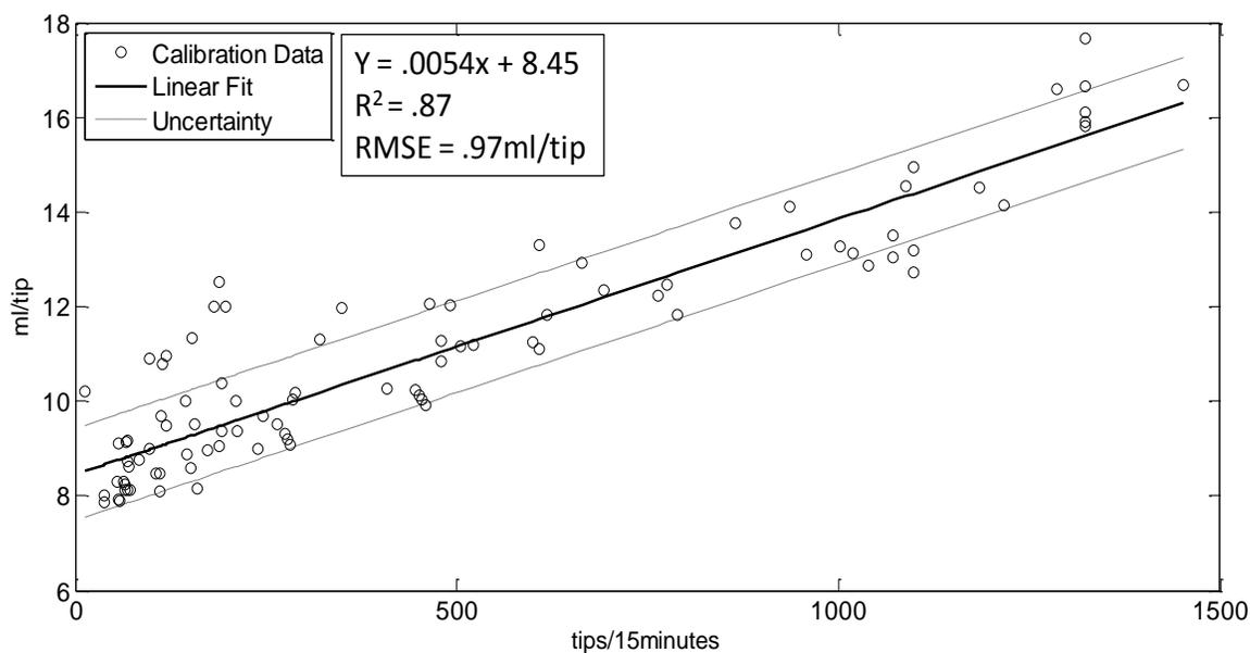
**Figure 5. Tipping bucket calibration data.**
