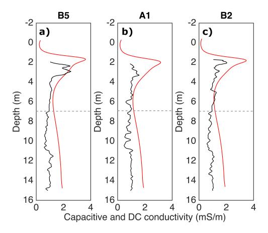
Figure 12: Recovered ER (with our method - in red) and capacitive conductivities (black) at borehole locations in the BHRS. The dashed gray line shows the cut-off for our appraised solution. Below the cut-off the solution returns to the reference model.
