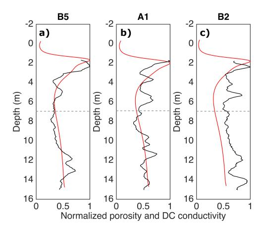
Figure 11: Normalized recovered conductivities (red) and borehole neutron porosity (black) at borehole locations in the BHRS. The dashed gray line shows the cut-off for our appraised solution.
