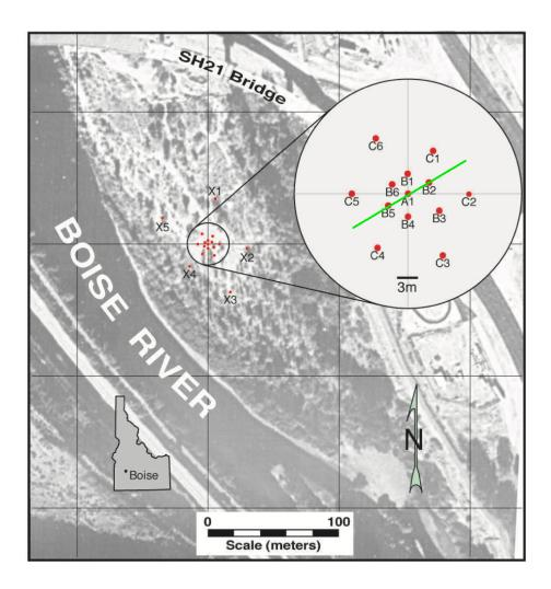
Figure 6: Geographic location of the Boise Hydrological Research Site (BHRS). The red dots denote the existing boreholes. Our survey line crossed boreholes B5, A1 and B2 as shown by the green line.
