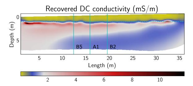
Figure 9: Recovered conductivity from the BHRS with topographic correction. The river is located towards the beginning of the survey line. The dashed cyan line represents the water table depth as measured on site (1m deep). The solid cyan lines represent the borehole positions. Note the higher conductivity, sand filled paleo channel that deepens toward the river. The pixel size is 0.05m on each side.
