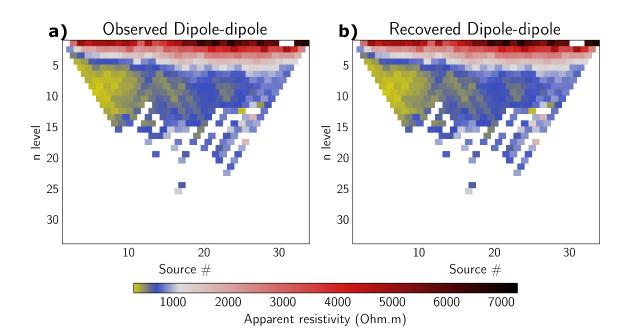
Figure 7: Dipole-dipole pseudo section with a-spacing equal to 1m from the BHRS.
