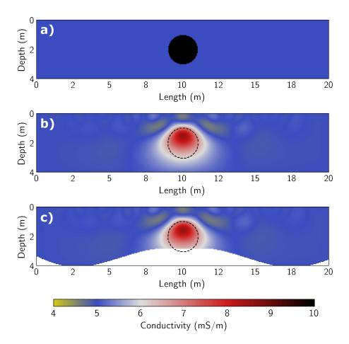
Figure 5: True  $\mathbf{a}$ , recovered  $\mathbf{b}$  and appraised  $\mathbf{c}$  conductivity for the synthetic example. The dashed cyan line represents a borehole location. The dashed black line represents the contour of the cylinder. The pixel size is 0.05m on each side.
