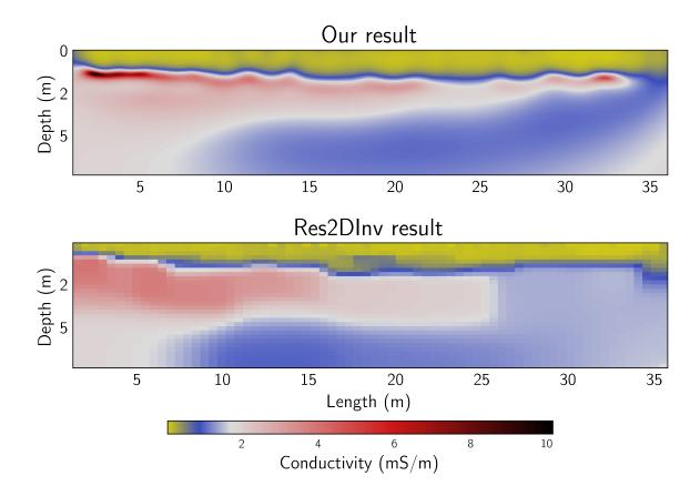
Figure 13: Comparison of our result in **a** and that of the commercial Res2DInv software in **b**. Results are shown in the computational domain without applying a topographic correction. The grid-size for **a** is 0.05m in width and length, while for **b** it is 0.5m long by 0.25m wide. The smallest possible horizontal spacing in Res2DInv is half of the receiver spacing (in this case 0.5m).
