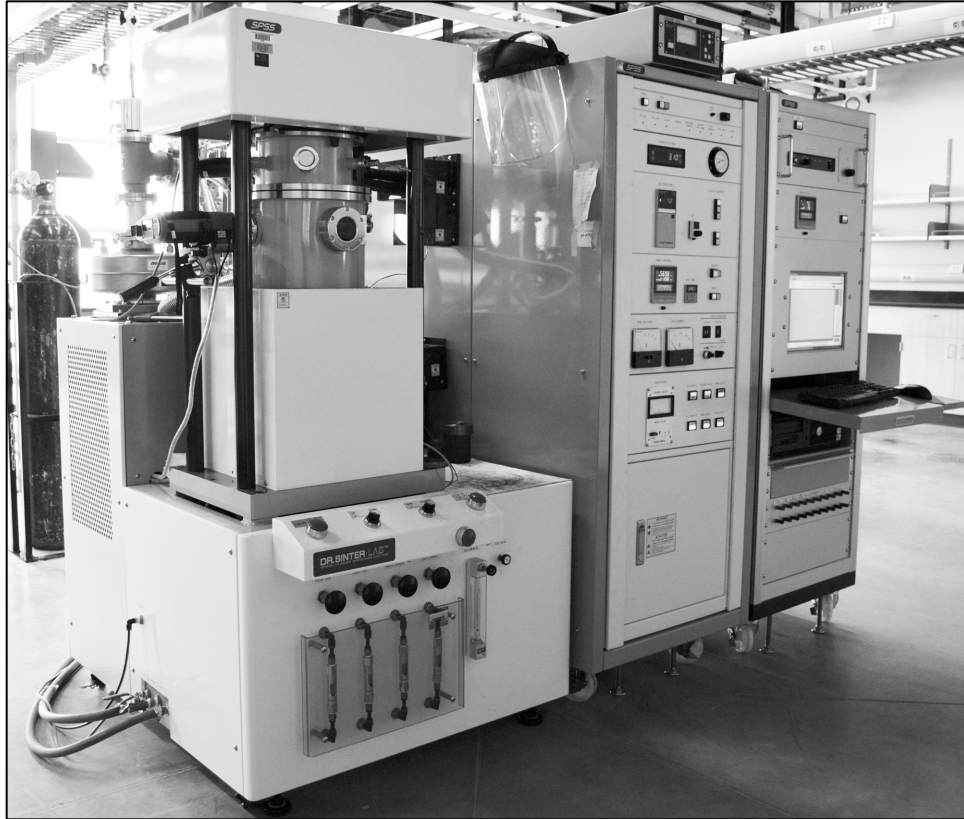
Figure 3.3. Dr. Sinter Lab SPS-515S spark plasma sintering unit located at the Center for Advanced Energy Studies. The infrared thermometer and sintering chamber are located on the left; the temperature controller, atmosphere control, and direct current generator are located in the middle unit; the data acquisition and pressure controls are located on the right unit.
