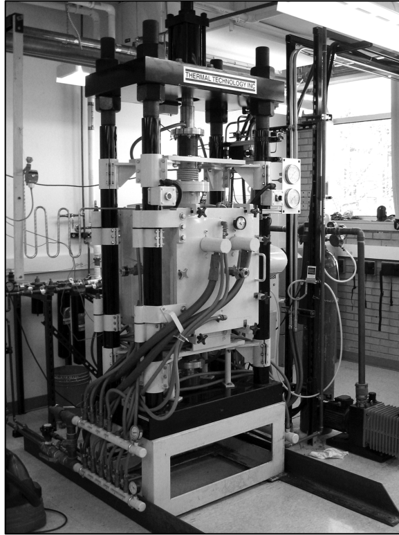
Figure 3.6. Thermal Technologies Inc. hot press located at Colorado School of Mines. Pure tungsten and W-4CeO 2 powders were hot pressed between 1300 and 1600 °C with an applied pressure of 42 MPa.
