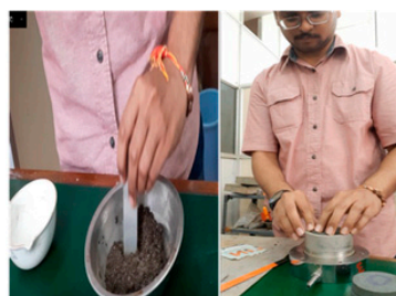
Following the dry mixing of chitosan and soil, the optimum moisture content is added and mixed uniformly. The homogeneously mixed sample is placed in the consolidation cell.
