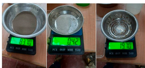
Oven dried soil, chitosan along with optimum moisture content are taken.
