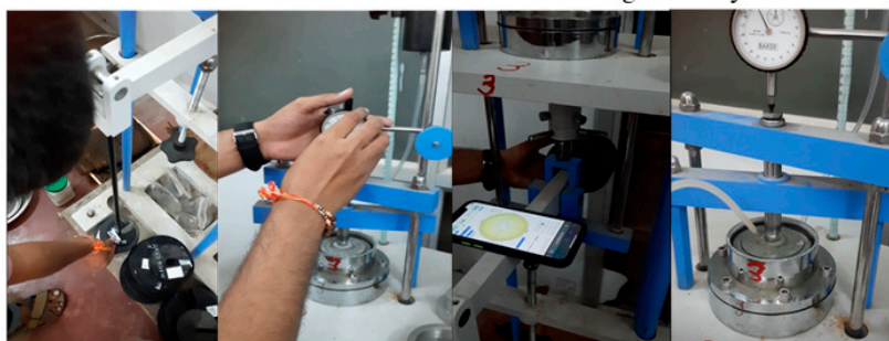
The consolidation cell is placed in the apparatus and subjected to saturation. Once the lever is made horizontal and the dial gauge is set to zero, seating load is applied.
