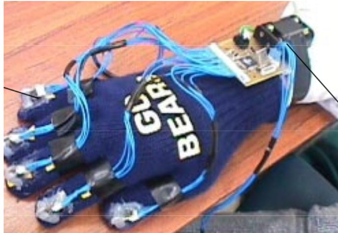
**Figure 1.9: Acceleration Sensing Glove[24]**
