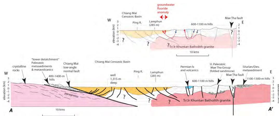
**Figure 4.** Structure cross section of the Chiang Mai basin modified after Morley et al. (2011). Fault locations are partly based on proprietary seismic and not exact. Upper picture shows a conceptual flow path (in red lines) of geothermal water and fluoride rich groundwater. Location of section in Figure 2.
