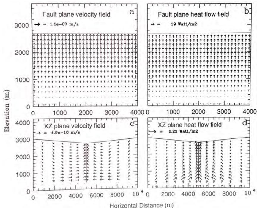
**Figure 5.** Diagram of flow in mountain block modeled by Lopez and Smith (1995). Mountain block has 300-m of relief above valley, and mountain block permeability is  $10^{-16}$  m<sup>2</sup> permeability— a (upper panel) is water flow in the 10-m wide fault plane, and a (lower panel) is water flow in the mountain blocks. b is heat flow.
