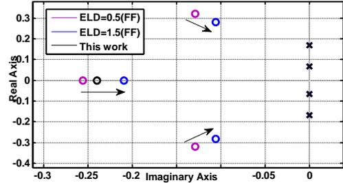
Figure 5. Pole-zero plot of  $FF(j\omega)$  and  $FF_{new}(j\omega)$  for CT- $\Delta\Sigma$  compensated for  $ELD = 0.5$  and  $1.5$ .
