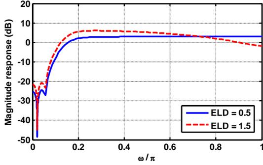
Figure 2. Comparison of  $NTF(e^{j\omega})$  and  $NTF_{new}(e^{j\omega})$ .
