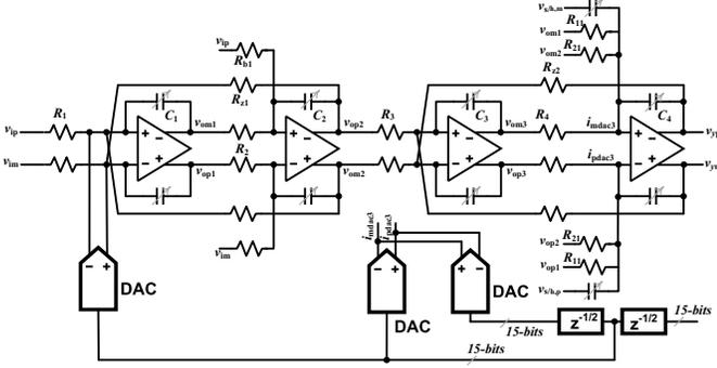
Figure 7. CT- $\Delta\Sigma$  modulator architecture.
