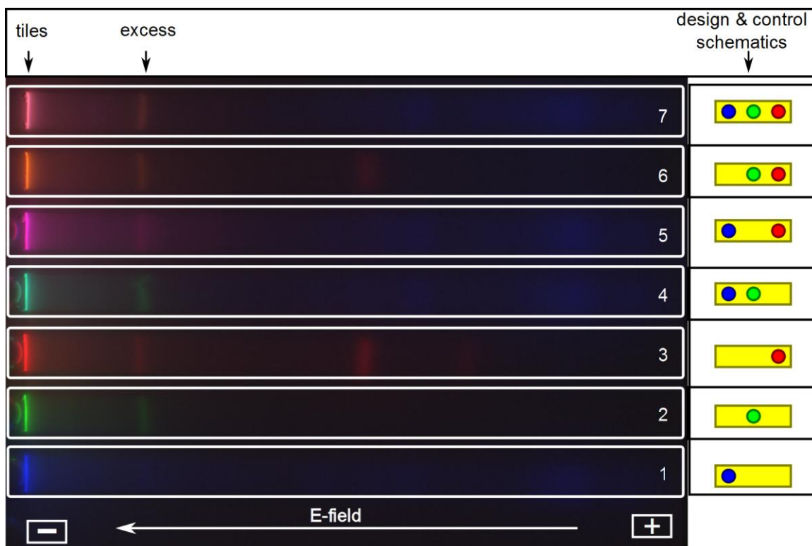
Fig.B.1: 10% PAGE gel in 1x TAE Mg^{2+} dye-labeled DNA tiles with (1) FAM, (2) TAM, (3) Cy5, (4) FAM-TAM, (5) FAM-Cy5, (6) TAM-Cy5, and (7) FAM-TAM-Cy5
