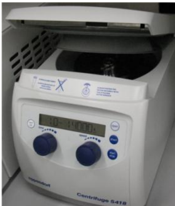
Fig.F.1: Eppendorf Centrifuge 5418, used for filtering DNA solutions
