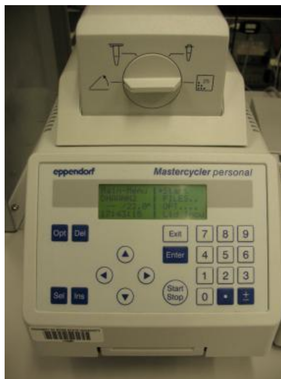
Fig.F.2: Eppendorf Mastercycler Personal, used for annealing DNA solutions
