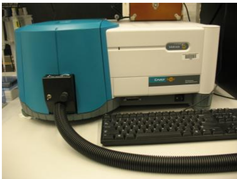
Fig.F.4: Agilent Varian Spectrophotometry, used for measuring fluorescence
